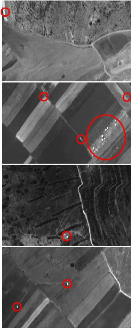
Fig. 5. Ground truth. A 30th-band of each one of 4 image cubes used for evaluation. The ground-truth anomalies were manually identified, marked in white and encircled in red.
